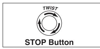
Figure 15. Resetting the STOP button.
